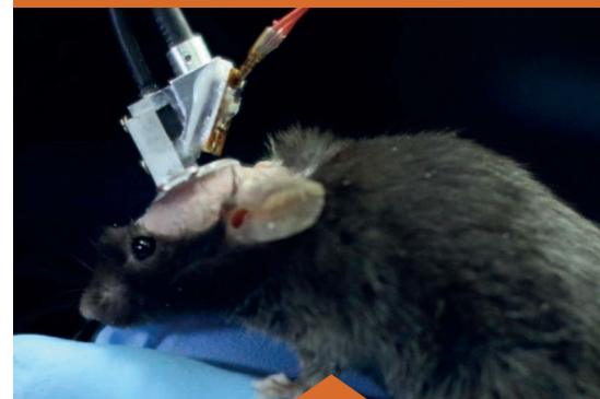
Cheng Heping's high-resolution, fast, miniaturized two-photon microscope enables imaging of neuronal structures in moving animals.
