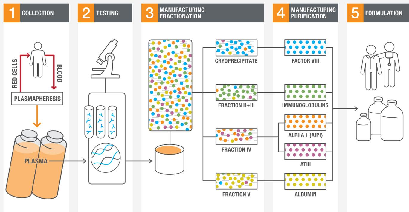
Figure 2. Manufacturing process for plasma-derived medicines.
